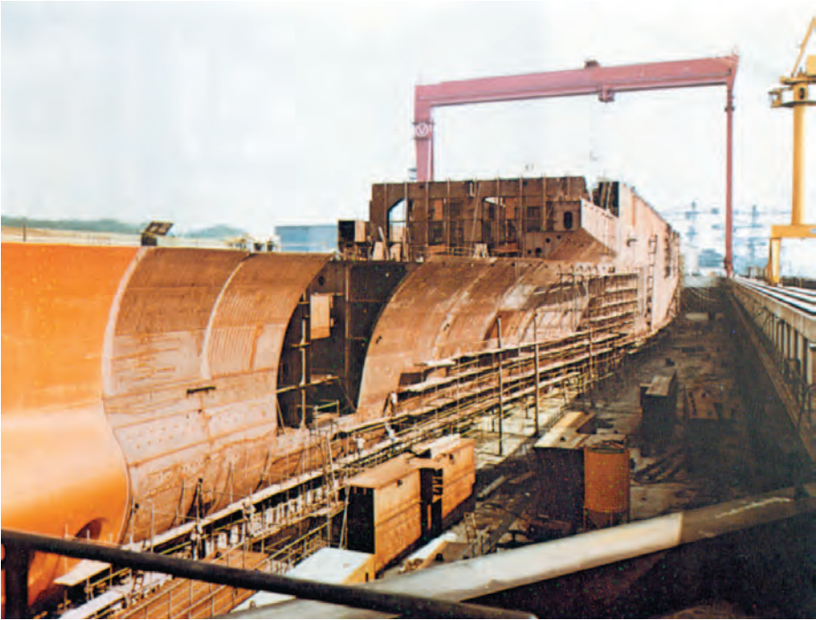
Assembly of a super tanker in the building dock.
