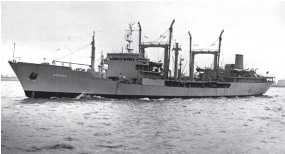
Turbine tanker equipped to refuel ships at sea.
