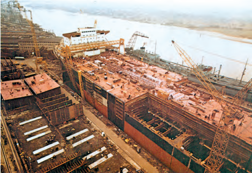
Assembly of a super tanker in the building dock.
