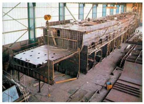
No. 1 Frigate under construction in Assembly Hall
