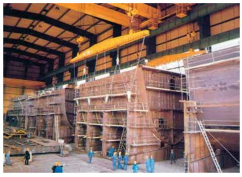
First big section almost completed for descaling and coating
