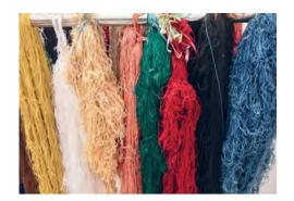
**Cotton** fibre is the most famous vegetable fibre. It is used in the textile industry. Cotton is stronger than wool. Warps and wefts are mainly made of cotton, but it can not be used for piles of carpet.
