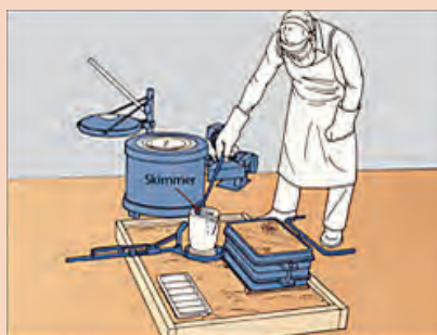
Skimming Slag from Molten Metal .....
