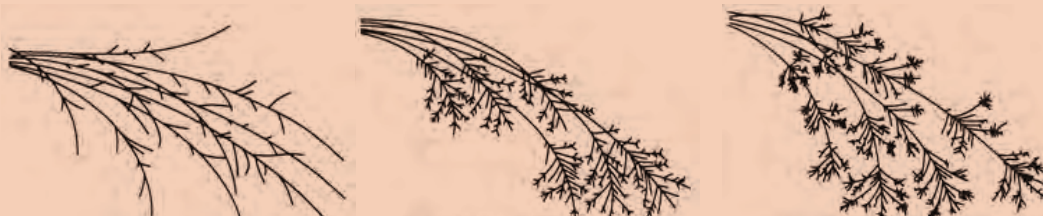
(a) Sparks from 1015 steel (0.15% C). (b) Sparks from 1045 steel (0.45% C). (c) Sparks from 1095 steel (1.0% C)
