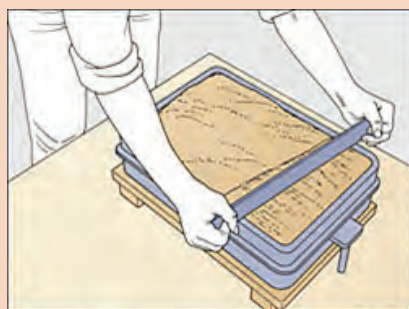
Level the Sand in the Drag .....
