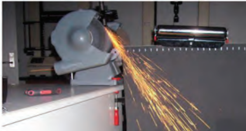
Figure 2: Spark test of a high carbon steel
