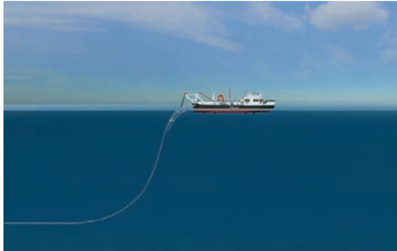
pipe laying vessel
