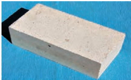
a heavy and dense refractory brick
