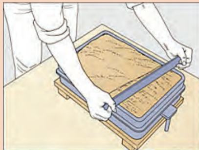
Level the Sand in the Drag .....
