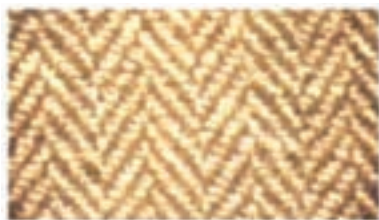
Herringbone twill in the opposite direction (zig zag effect)
