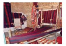
In fact the color and design of Jajim is dependent on color of wraps. The colors and designs of warps are chosen from the beginning of the process of wrapping. The color of warps cannot be changed. Therefore this limits the designs of Jajim.
