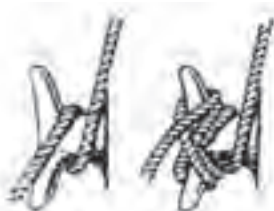
Belaying a rope to a cleat
