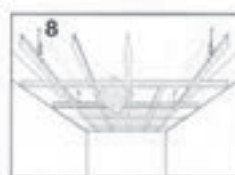
8.Installation of field and service tiles
