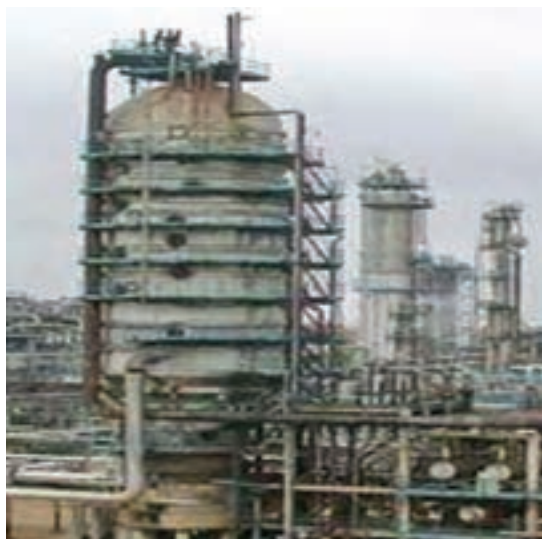
Fig. 20: Vacuum distillation tower
