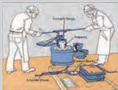
Removing a Crucible from a Furnace .....
