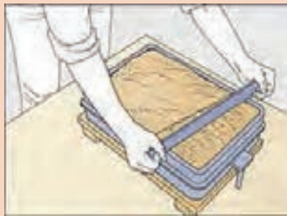
Level the Sand in the Drag .....
