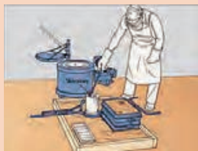
Skimming Slag from Molten Metal .....
