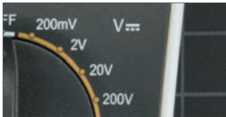
Use the V with a straight line to measure DC Voltage
