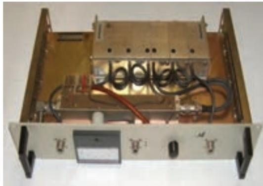
**Figure 20– Duplexer (Tx/Rx switch)**
