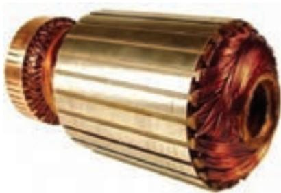
Figure 10 - Armature of a DC motor
