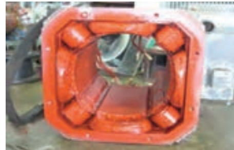
Figure 11- Stator of a DC motor
