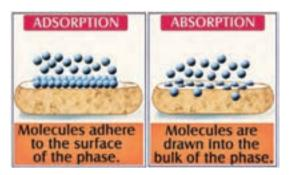
Fig 6: Adsorption and absorption
