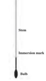
Fig. 25: A stem - type thermometer
