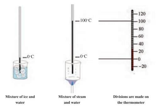
Fig. 27: Thermometer calibration
