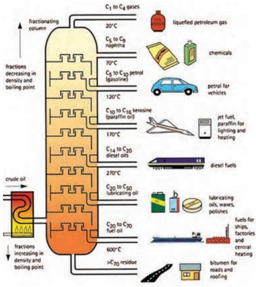
Fig. 19: Distillation of crude oil
