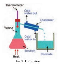
Distillation processes are widely used for the separation of organic chemicals and for the separation of gases, usually at cryogenic temperatures, as in the production of oxygen and nitrogen from air (Fig.3).
