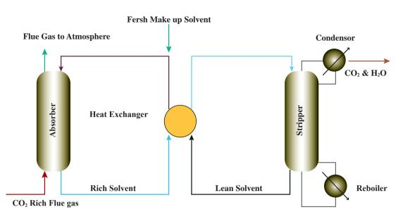
Fig.7: Absorption and stripping
