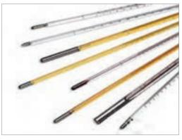
Fig. 26: Laboratory liquid - expansion thermometer
