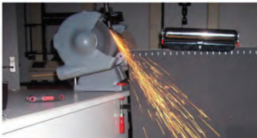
Figure 2: Spark test of a high carbon steel
