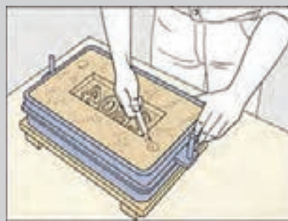
Cutting the Gates .....
