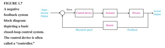
to the right, the rudder is actuated to direct the ship to the left. The system shown in Figure 1.7 is a negative feedback control system, because the output is subtracted from the input and the difference is used as the input signal to the power amplifier.
