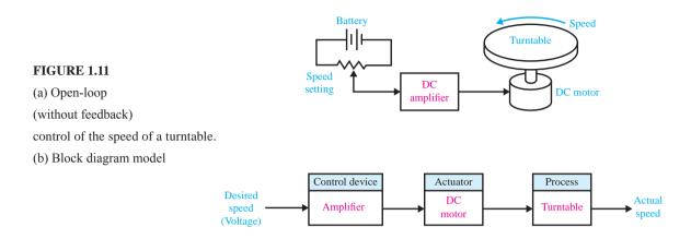
To obtain disk rotation, we will select a DC motor as the actuator because it provides a speed proportional to the applied motor voltage. For the input voltage to the motor, we will select an amplifier that can provide the required power.
