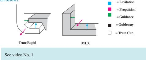
**Levitation:** Levitation is the ability for the train to stay suspended above the track. There are two important types of levitation technology:
