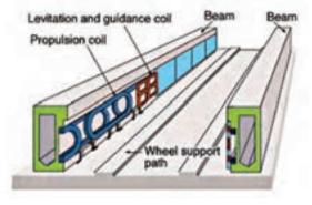
Magnetized coils run along the track called a guide-
