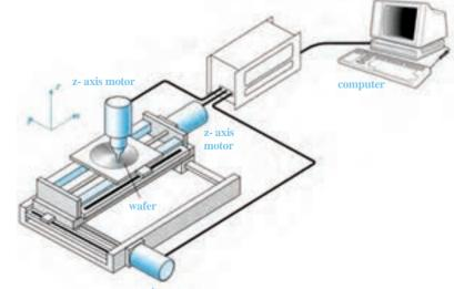
FIGURE 1.8 A three-axis control system
