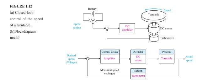
We expect the feedback system of Figure 1.12 to be superior to the open-loop system of Figure 1.11 because the feedback system will respond to errors and work to reduce them. With precision components, we could expect to reduce the error of the feedback system to one-hundredth of the error of the open-loop system.
