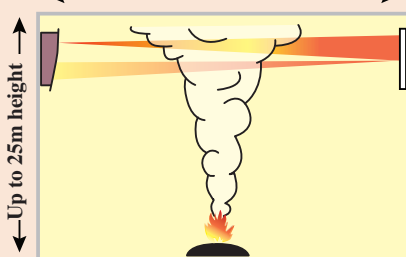
operation of reflective type optical beam smoke detector
