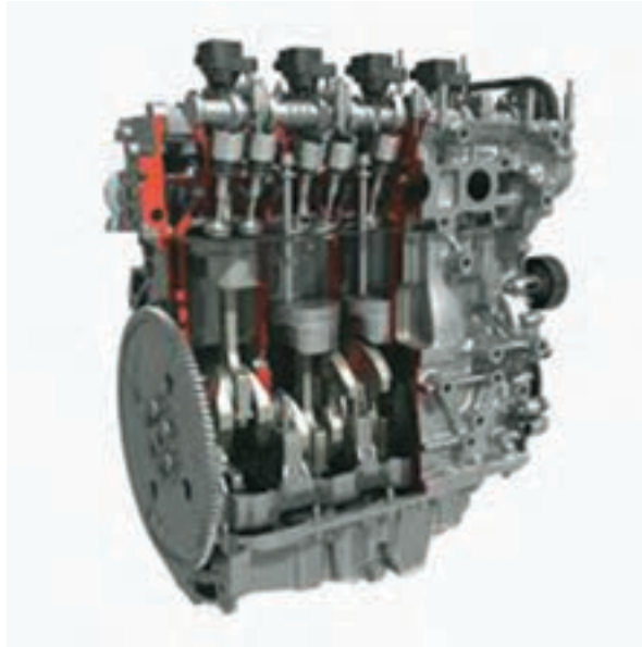
Fig 24: A four-Stroke Engine
