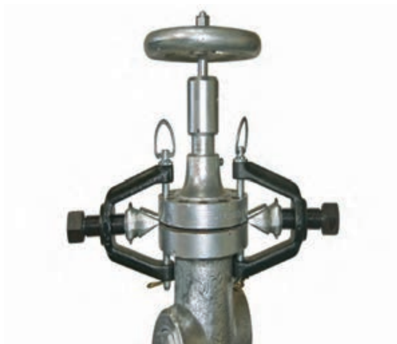
Fig 19: A flange splitter
