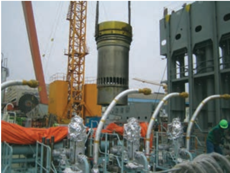
Fig 27: Big engine cylinder liner
